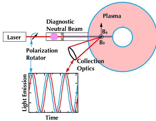
FIG. 2. MSE-LIF setup for pitch angle measurement on the toroidal confinement device.
