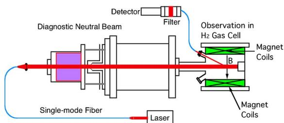
FIG. 3. MSE-LIF development laboratory setup.
